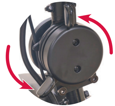
EZ Pivot Tiller System That Can Be Adjusted By Hand or Foot
